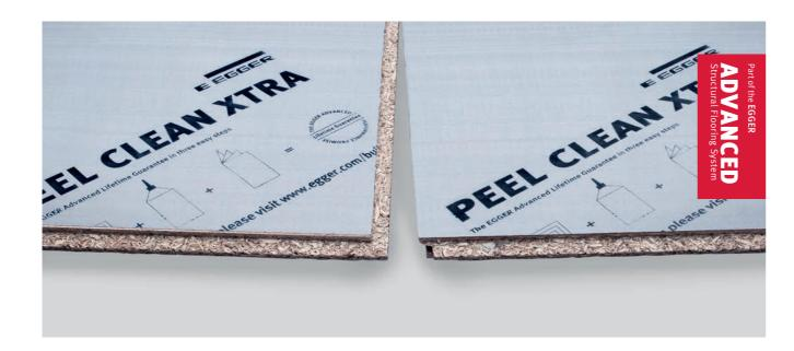
Made from EGGER P5 grade chipboard, this robust product is covered with an easy-to-peel, anti slip polyethylene film which helps to prevent moisture ingress during the build process.
